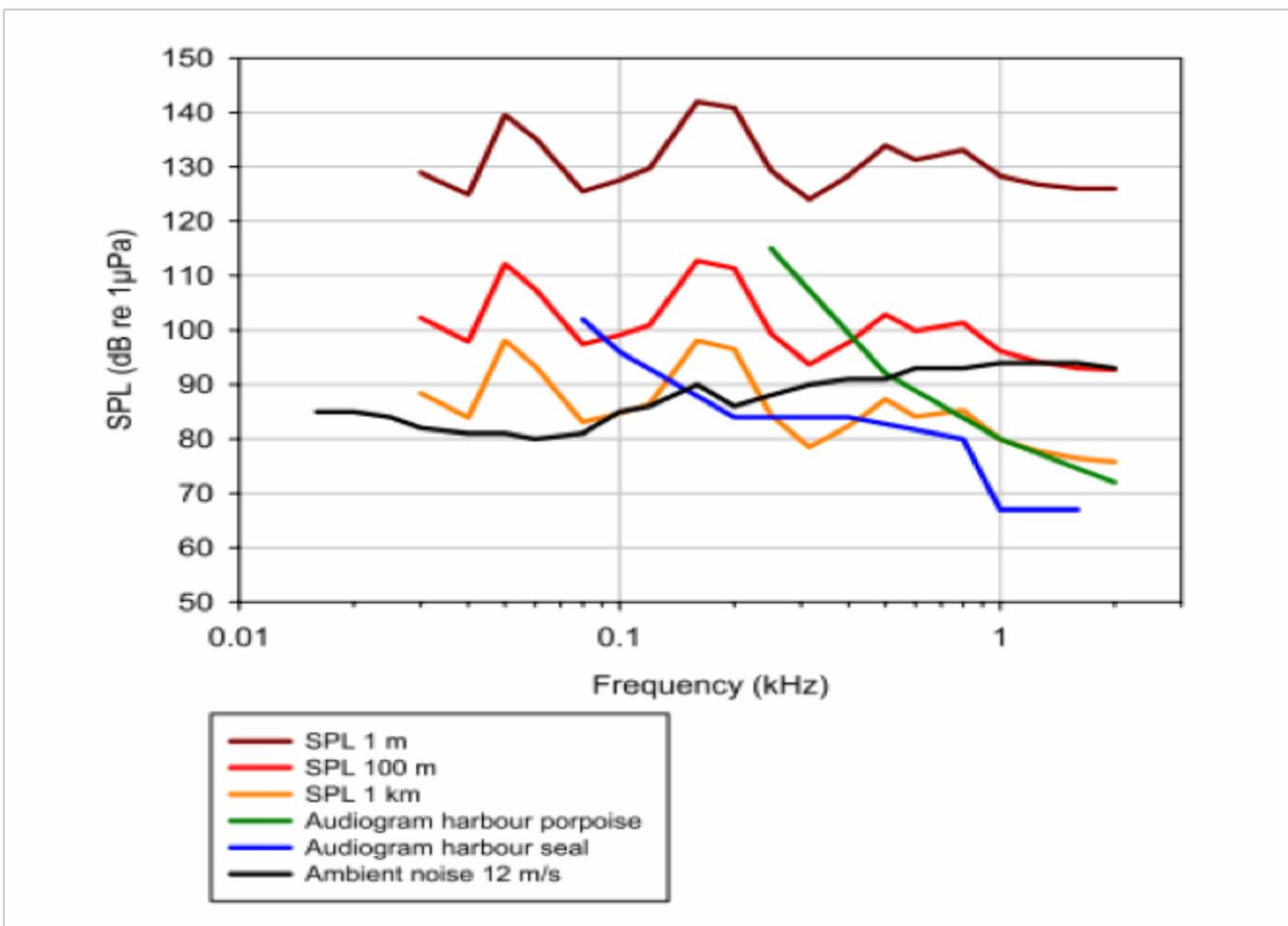
**Figure 2:** Sound pressure levels of offshore wind farm in operation at different distances from the source compared to the audiogram of harbor porpoises, harbor seals, and ambient noise. Measured by sound pressure level (SPL) given in decibels (dB) at the different frequency levels measured in kilohertz (kHz). At 100-meter distance, turbine noise would be
