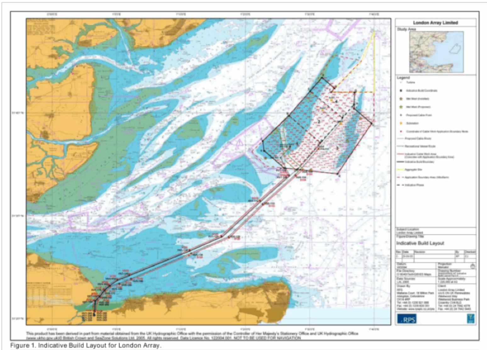
**Figure 1:** The planned layout of the London Array. The location within the London Estuary of the proposed wind farm is shown along with the layout of the four phases, each planned wind turbine, and the cable route (London Array Consents Manager, 2005).
