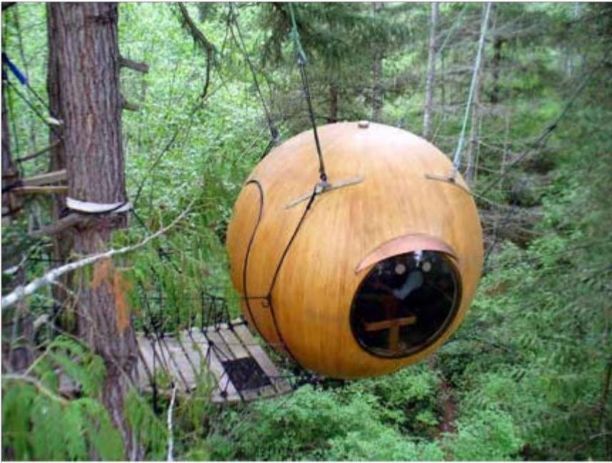
Figure 3. Free Spirit Sphere hanging in the rainforest in Vancouver Island, Canada. Note the number of tether points as well as the ropes connecting the “sphere” to other parts of the rainforest in order to suspend it, providing the Free Spirit Sphere with strength (Nellemann, 2009).
