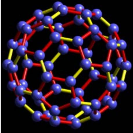
Figure 1-2: Shows a single-bond ball and stick model of Buckminsterfullerene ( $C_{60}H_{60}$ ). Each of the blue balls represents a carbon. It is difficult to count but there are 12 pentagons and 20 hexagons present. Buckminsterfullerene follows principle #2 of the “rules-to-build-by” (Morris, 2010) <http://www.godunov.com/Bucky/buckyball-2.gif>
