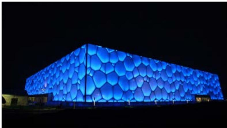
Figure 1: This is an image of the outside of the Beijing National Aquatics center. As can be seen this building is composed of many different cells linked together, giving the building a look similar to bubble in a foam
