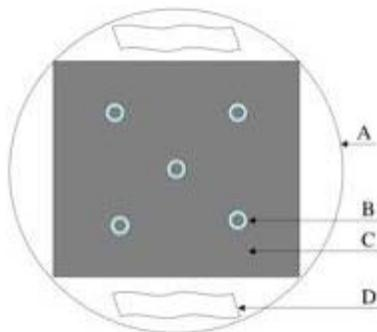
**Fig. 1.** Humidity chamber containing coverslip pedestals. (A) Large Petri dish. (B) Coverslip pedestal fabricated from eppendorf tube caps. (C) Sheet of parafilm. (D) Kimwipe soaked in water. Each humidity chamber includes an opaque cover.
