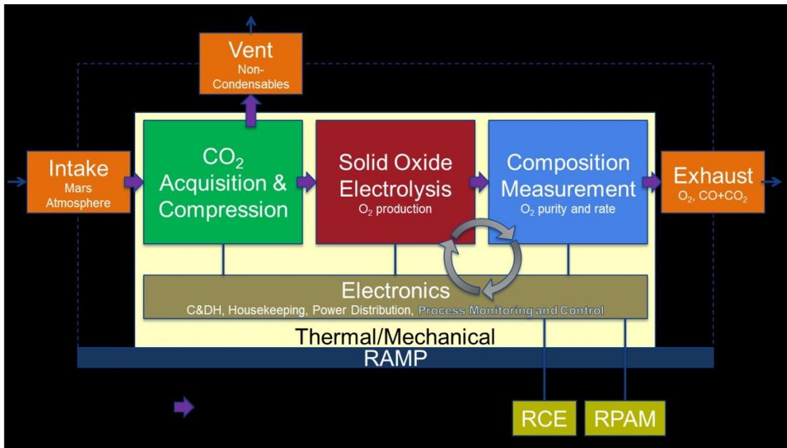
*Figure 3. MOXIE Functional Block Diagram. This image represents the mechanism involved in MOXIE in order to take in carbon dioxide from the atmosphere and convert it to oxygen and other gases. Figure adapted from “The Mars oxygen ISRU experiment (MOXIE)” by M. Hecht, D. Rapp, and J. Hoffman, 2015. Copyright 2015 by the M.I.T. Dept. of Aeronautics and Astronautics. Retrieved from: <http://mars.nasa.gov/mars2020/mission/science/for-scientists/instruments/moxie/>*
