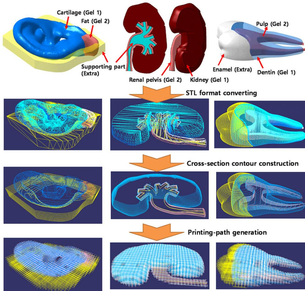
**Figure 1.** *The Process of Generating Printing Paths.* From left to right, outer ear, kidney and tooth images that are the results of slicing algorithm and the algorithm to generate printing paths. The frame is shown in white, hydrogel 1 in blue, hydrogel 2 in red, and the support in yellow. Figure adapted from Jung, Lee & Cho, 2016.
