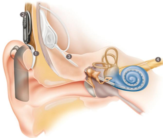
**Figure 1.** 1 is speech processor. 2 is transmitter. 3 is internal implant. 4 is auditory nerve. The electrode array is placed inside the cochlear (blue area). This figure is originally from webpage of cochlear.com (Cochlear.com, n.d.). Available at <http://www.cochlear.com/wps/wcm/connect/au/home/understand/hearing-and-hl/hl-treatments/cochlear-implant>
