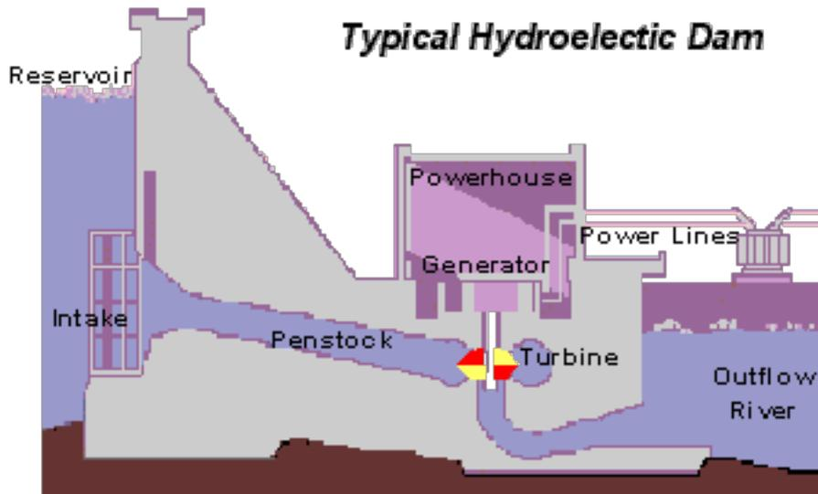
Figure 2: Different components of a hydropower plant. The reservoir stores water and the penstock is where the water flows down and turns on the turbine and the generator creates electricity. Hydropower plants generate electricity from the buildup gradient of water going down the penstock due to gravitational pull (*figure from Perlman, n.d*).
