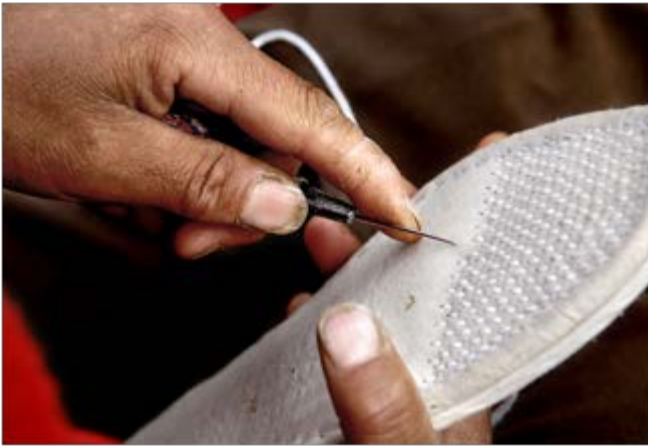
Figure 4 A close-up photograph of a shoemaker sealing shoe sole pads. Cottons and other fabrics are sandwiched between shoe pads, and sealing the pads starts from sealing the edges. Thick needles and twines are used to seal up the pads.
