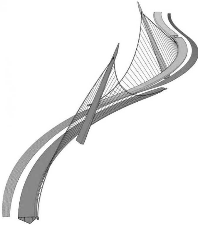
Figure 4: Dimeric Architecture of The Peace Bridge. Architectural design of the Peace Bridge, by Wilkinson Eyre. The bridge is constructed from two identical suspension half-bridges, each spanning half of the river. The half-bridges meet in the middle to create a whole bridge for passage across the River Foyle. (Retrieved from WilkinsoEyre, https://www.wilkinsoeyre.com/projects/the-peace-bridge ).
